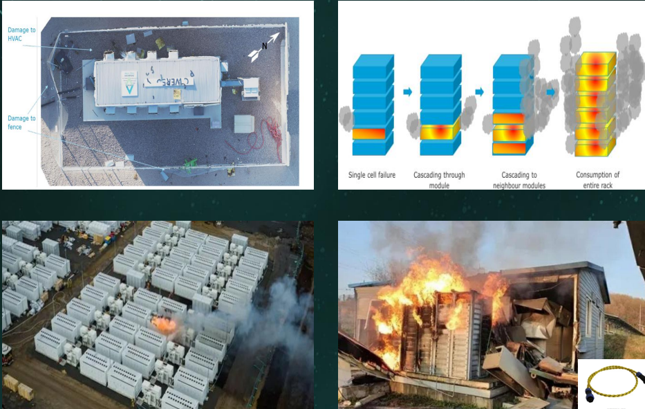
Figure 1. Aerial view of Damaged APS BESS (2019); DNV investigated Report for APS' s TR hazards; Victorian Big Battery failure (2021); One Korean NCM BESS station caught on fire; coolant leakage detector with a leakage detector (clockwise)
