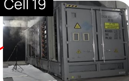
(e) Cell 19 Thermal runaway [01:01:07]
