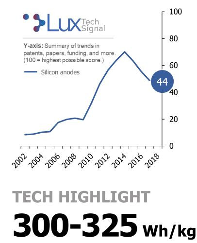
Leading startups claim that cells with their silicon-carbon composite anodes achieve more than 300 Wh/kg and 1,000 cycles to 80% depth of discharge.
