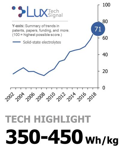
Solid-state batteries incorporate solid electrolytes as well as metallic lithium anodes; thus, they offer both improved energy density and improved safety over incumbent Li-ion cells.
