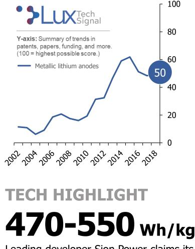
Leading developer Sion Power claims its cells with conventional lithium foil anodes achieve 470 Wh/kg and its cells with its proprietary protected lithium anodes achieve 550 Wh/kg.
